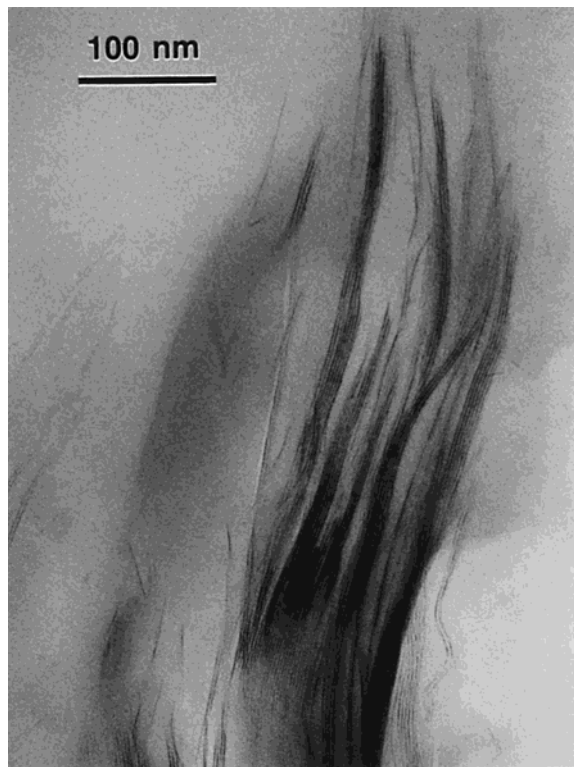
Figure 6. TEM of an intercalated tactoid ( d spacing 3.5 nm) of PPgMA-layered-silicate (mass fraction 4%) nanocomposite.
