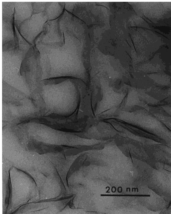
Figure 7. TEM of the combustion char from the PPgMA-MMT nanocomposite (4%) showing the carbonaceous-silicate multilayered structure.
